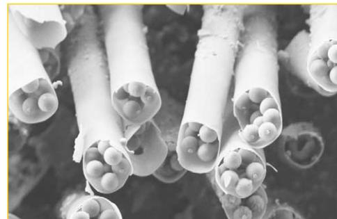
Colloidal crystals within silica tubes, coated with metal to reduce charging during imaging. (© 2005 American Chemical Society.)
