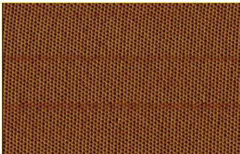
AFM image of a triblock copolymer thin film after removal of both the PMMA and PEO. (Courtesy of Craig J. Hawker.)
