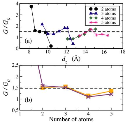
FIG. 5 (color online). (a) Evolution of the conductance of 2, 3, 4, and 5 atom chains as a function of  $d_z$  (circles, triangles, diamonds, and stars, respectively). (b) Conductance vs the number of atoms in the chain measured at the equilibrium distance (crosses) and averaged over a range of 2 Å about such distance (squares).
