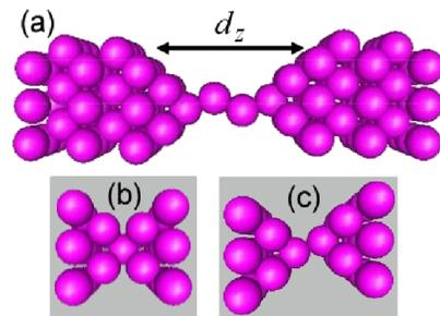
FIG. 2 (color online). The different chains connecting (001) oriented fcc leads studied in this Letter: (a) 4-atom chain, (b) single atom contact, and (c) 2-atom chain.  $d_z$  is the distance between leads.
